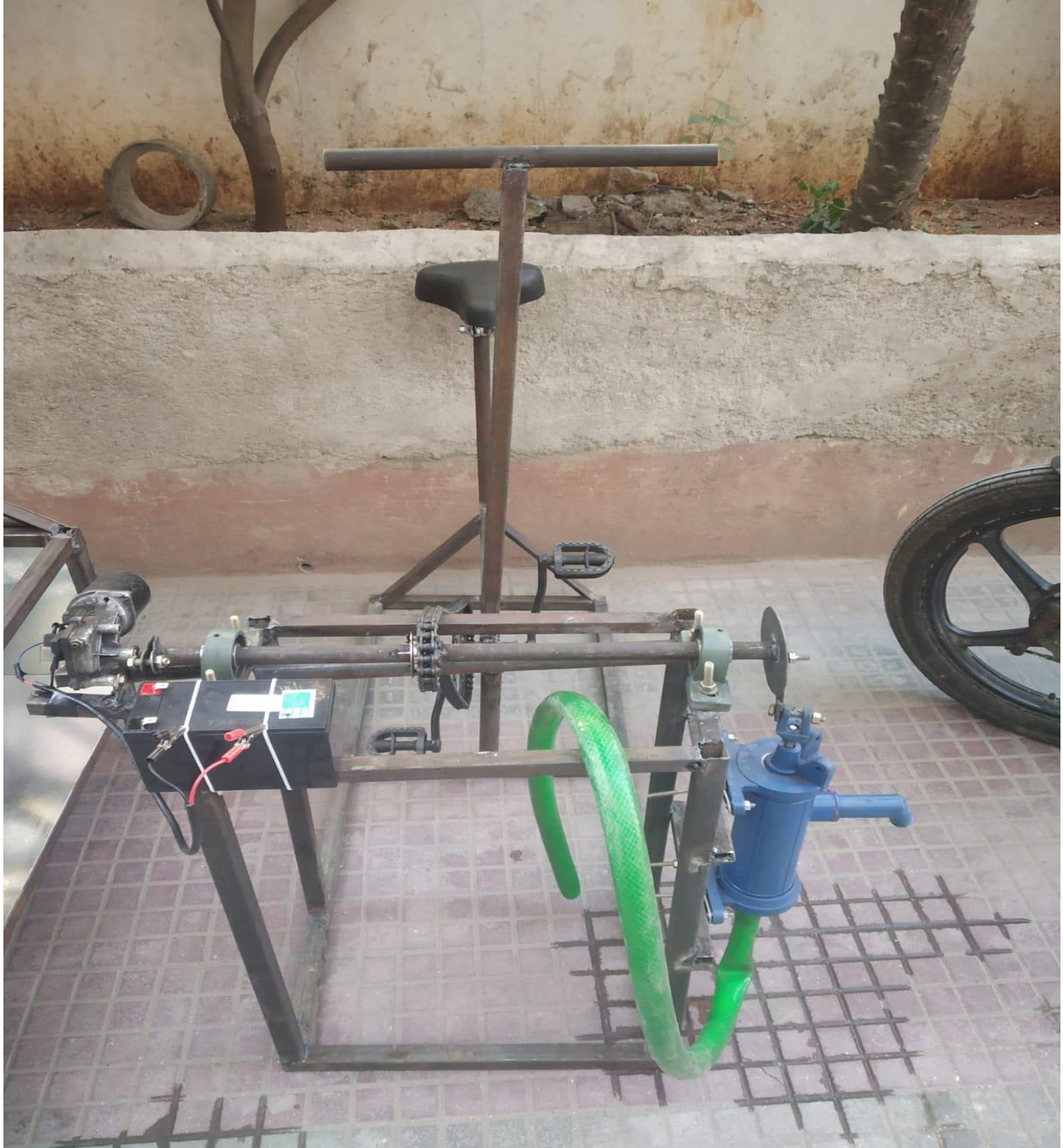
PEDAL AND MOTOR OPERATED WATER PUMP
